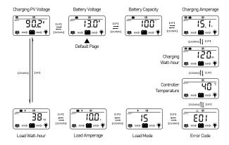
The battery voltage view will be displayed by default. Use the up and down arrow keys to cycle through different views. The battery voltage view will resume upon 30 seconds of inactivity. The error code view will be displayed when an error is detected. The backlight in the screen will be on for 20 seconds with any button operation.
